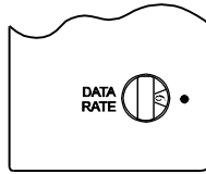
Data rate switch set to the default position 6 (2.5 Mbps).
